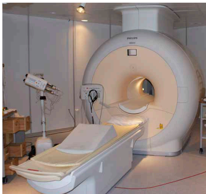
Magnetic resonance imaging (MRI) scanners use specialized magnets that require extremely low temperatures to operate. These low temperatures are achieved using liquid helium, which is the only currently available source of ultra-low cryogenic temperatures. Helium is sourced entirely from natural gas. Image credit: Jan Ainali, Wikimedia Commons. 24
