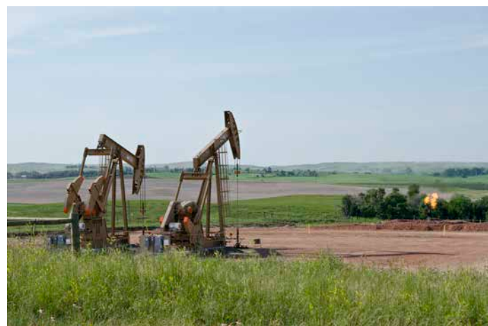
Flaring of unprocessed natural gas, as seen here on a well site in North Dakota (flare on right of picture), is one of several oilfield processes that can negatively affect air quality, as well as increasing carbon dioxide emissions. Flaring in North Dakota was particularly common in the early 2010s, as oil production was booming but pipelines were not in place to collect and transport the natural gas produced from oil wells. Image credit: Tim Evanson, Flickr. 3
