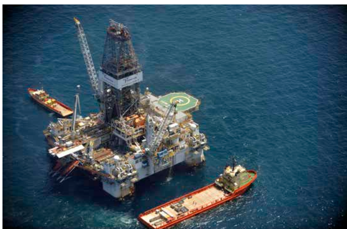
Transocean Development Driller drilling a relief well in the Gulf of Mexico to relieve the pressure on the leaking Macondo well, 2010. This rig can drill to depths of 37,500 feet in as much as 7,500 feet of water. Image credit: U.S. Coast Guard. 20
