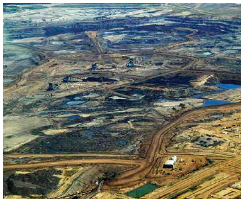
Open-pit mining of oil sands in Alberta, Canada. The ponds in the photo are “tailings ponds”, containing a mixture of water, fine sand, clay, and residual oil components after the sands have been processed to remove most of the oil. Image Credit: Dru Oja Jay, Dominion. 14
